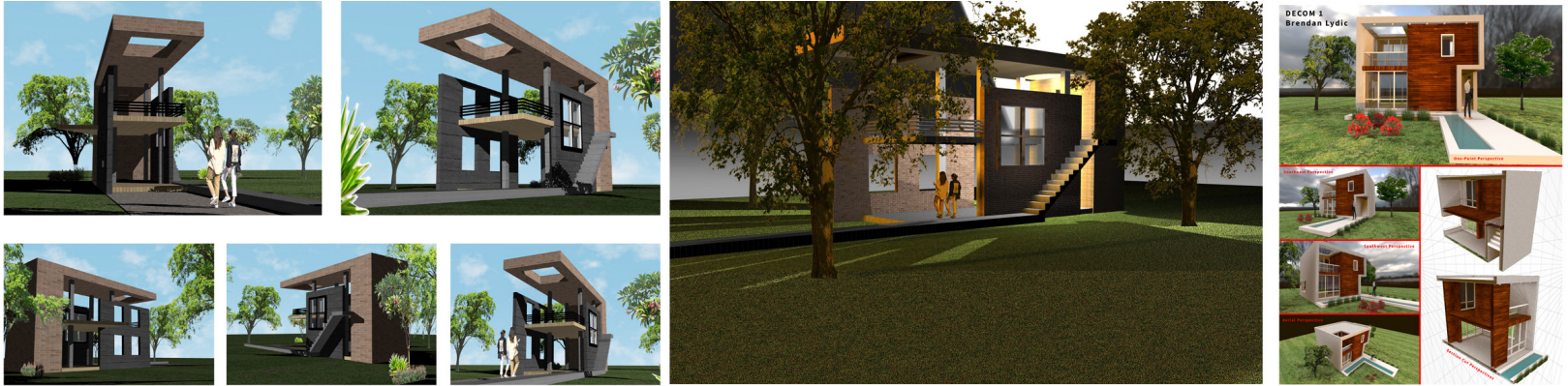
Design Communication I. Rhino for architectural 3D modeling, texture mapping, and rendering. Hand-drawn plan as underlay to create plan, section, elevation, and 3D using Rhino
